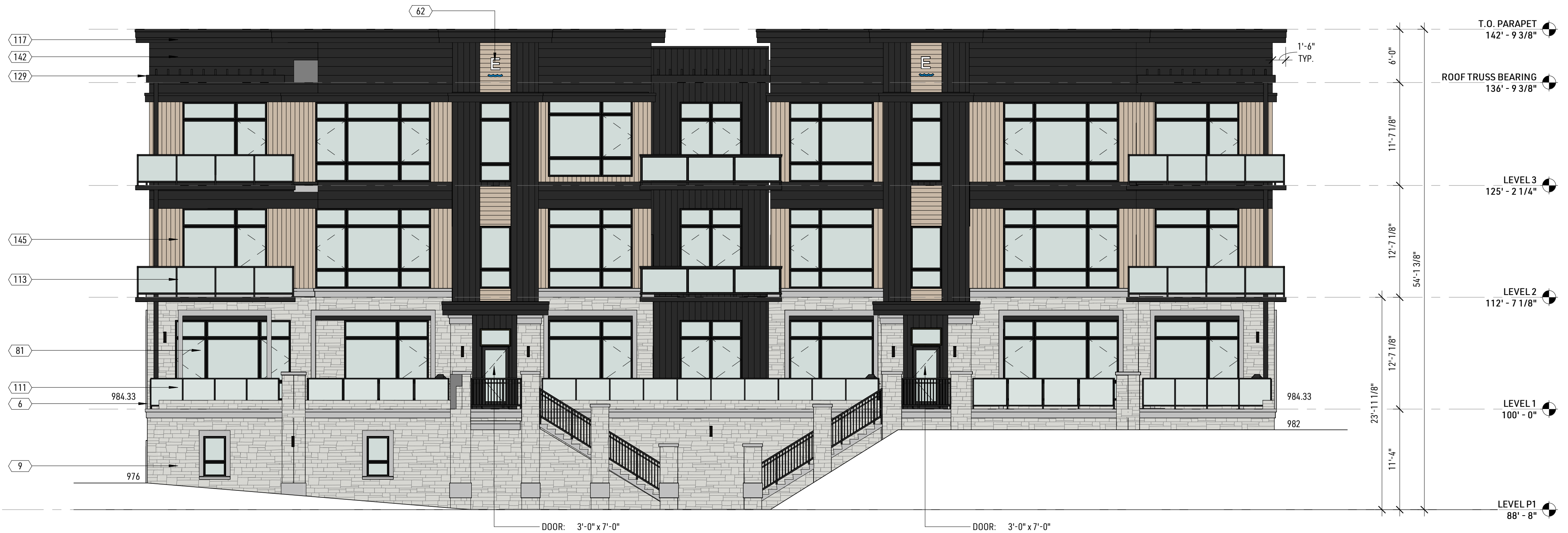
1 SOUTH EXTERIOR ELEVATION 1/8" = 1'-0"
